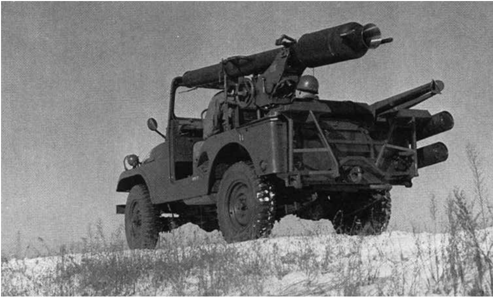
The Davy Crockett was capable of firing atomic or conventional warheads. Here it is shown in Jeep mounted mode in 1960.
