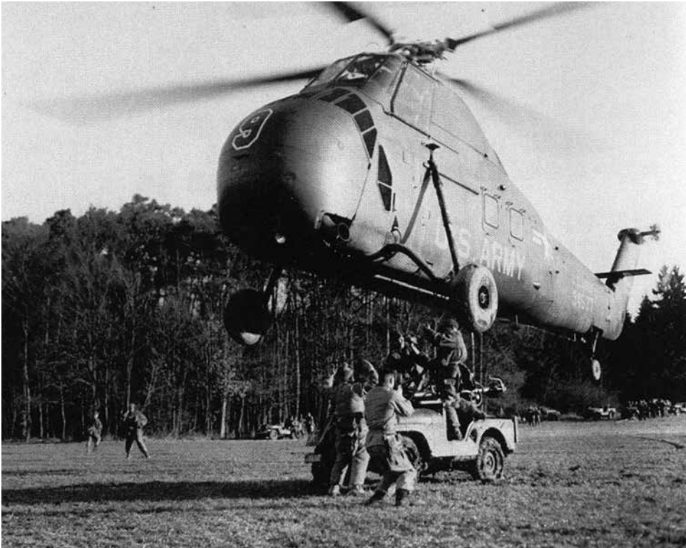
Soldiers of the 11th Airborne Division attach a ¼-ton jeep with recoilless rifle to an H-34 helicopter for air assault during Exercise SABRE HAWK.
